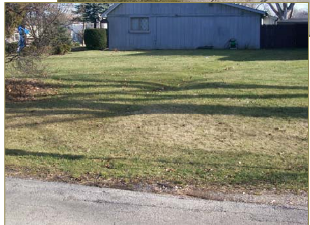
Addition of sidewalks and parkway grading for new curbs may block existing drainage such as the existing drainage patterns found on these lots between 168 and 152 and lot 145 on Henderson Street.
