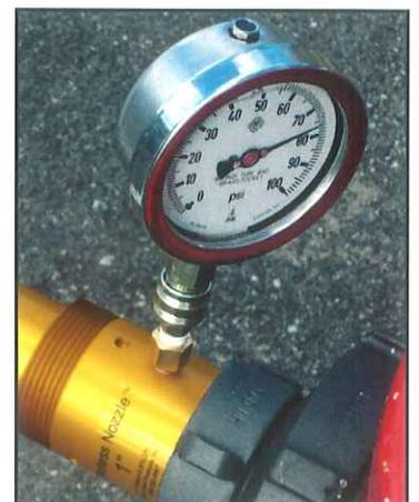
Pitotless nozzle for precise flow rate
