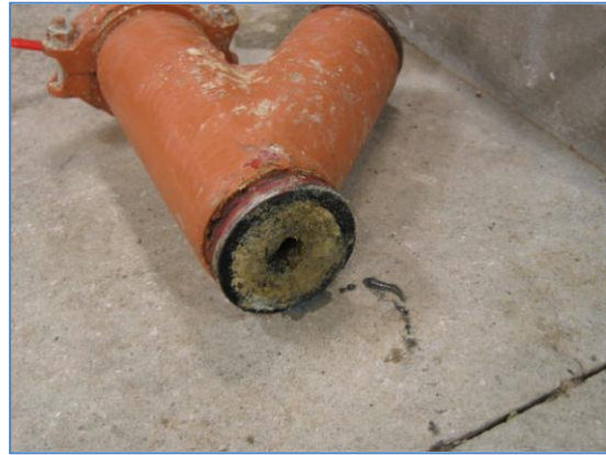
Grease almost closing inside pipe diameter
