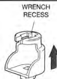
PUSH WRENCH IN TO ENSURE ENGAGEMENT WITH SPRINKLER WRENCHING AREA FIGURE 4 W-TYPE 7 RECESSED SPRINKLER WRENCH
