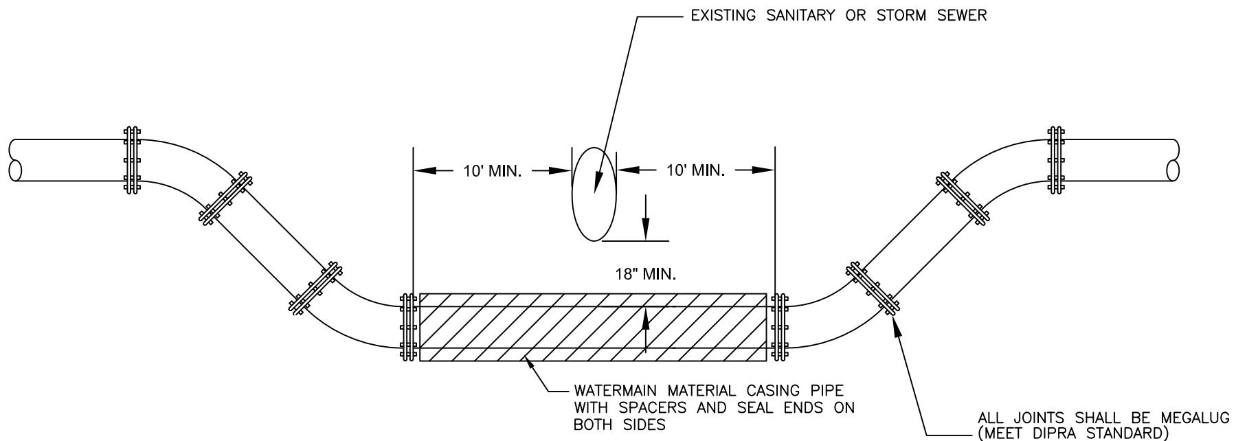
NOTE: ALL FASTENER HARDWARE (i.e. NUTS, BOLTS, AND WASHERS) ASSOCIATED WITH THE WATERMAIN AND CASING SPACERS SHALL BE STAINLESS STEEL.
